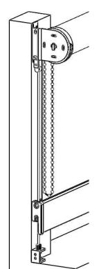
With the shade lowered all the way down, stretch the cable vertically to find the best position for the hold down bracket. Attached the U hold down bracket to the wall or a floor. Make sure the U brackets is vertically below the upper brackets and there are no obstacles between them.
