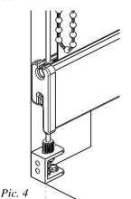
5. Lower and raise the shade making sure the cables are not binding and hem bar is sliding smoothly. Pic. 4
